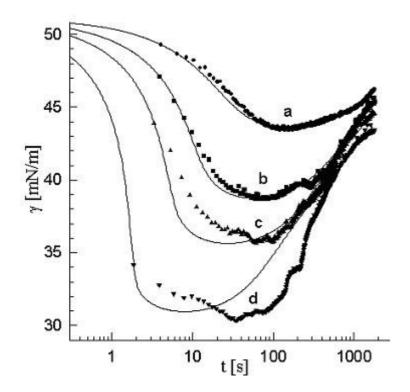
Dynamic interfacial tension during the adsorption and transfer of  $C_{13}$ DMPO at the water/hexane interface; the hexane phase is initially free from surfactant; water/hexane volume ratio is 10<sup>-3</sup> (single water drop in a hexane environment); initial concentrations in water:  $C_0=1.10^{-8}$ (a),  $2.10^{-8}$  (b),  $3.10^{-8}$  (c),  $5.10^{-8}$  mol/cm<sup>3</sup> (d)
