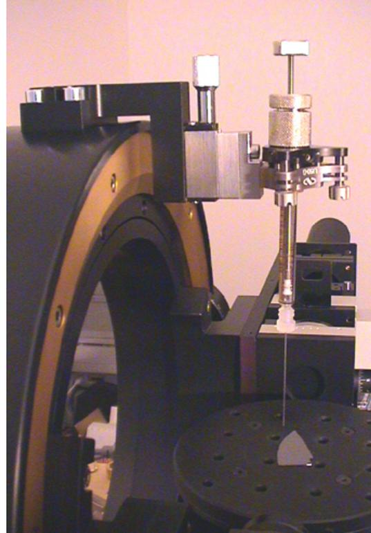
A contact angle measurement requires the precise determination of the location of the three phase contact point. Many commercial programs demand further user input to solve this task but not our program CAM. The implemented contour tracing algorithm automatically distinguishes between drop and mirror image. This is fast, accurate and user friendly.
