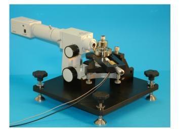
THE BUBBLEDROP ANALYZER of OPTREL GBR is a powerful surface analytical tool for Colloid and Interface Science. It measures the complex surface dilatational modulus E of aqueous surfactant solution in a frequency range of 1 to 600 Hz. The extension to the mid frequency range is decisive for the investigation of soluble surfactants as the molecular exchange processes between adsorbed and dissolved amphiphiles contribute at higher frequencies significantly to the E-modulus.
